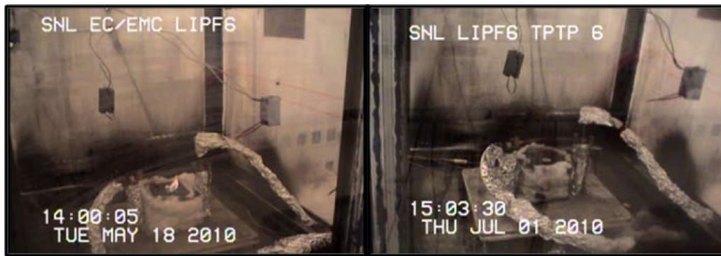
Photo 1. Shows that CAR-1 on the left is flammable and CAR-HFE-1 on the right is nonflammable.
